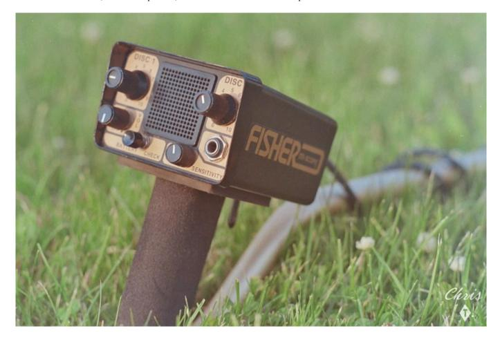
All types of metal are detected at the zero level while the most pieces of trash are rejected at ten.. If you walk too fast you can't overlap your sweeps and you'll miss a lot of ground.. "• DISCRIMINATION POINTS 8 Some objects will cause sharp static or "ticking" when rejected.
